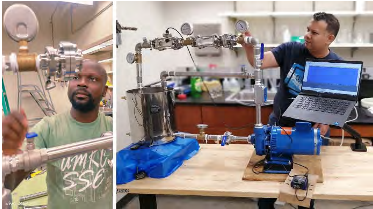
Figure 1 Researchers checking the cavitation system for leaks and functionality.
