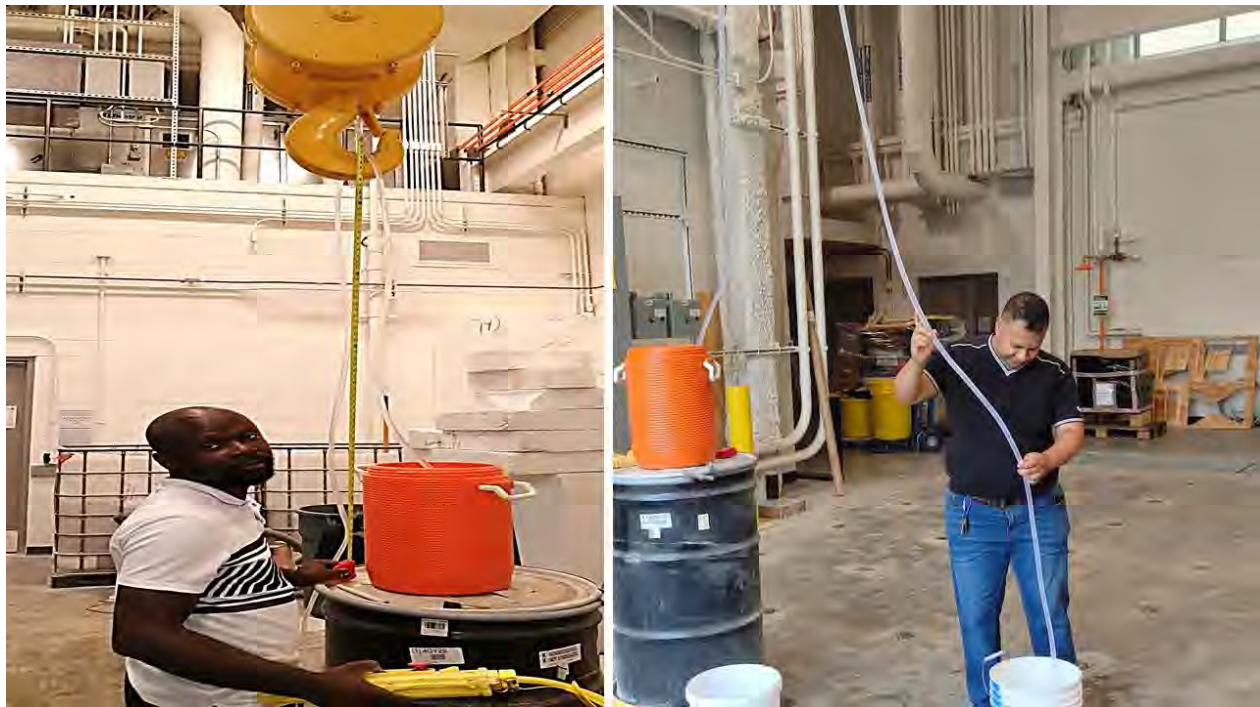
Figure 3 An attempt to demonstrate syphoning cavitation using the overhead crane, 16 mm pipe and two 25-litre buckets.
