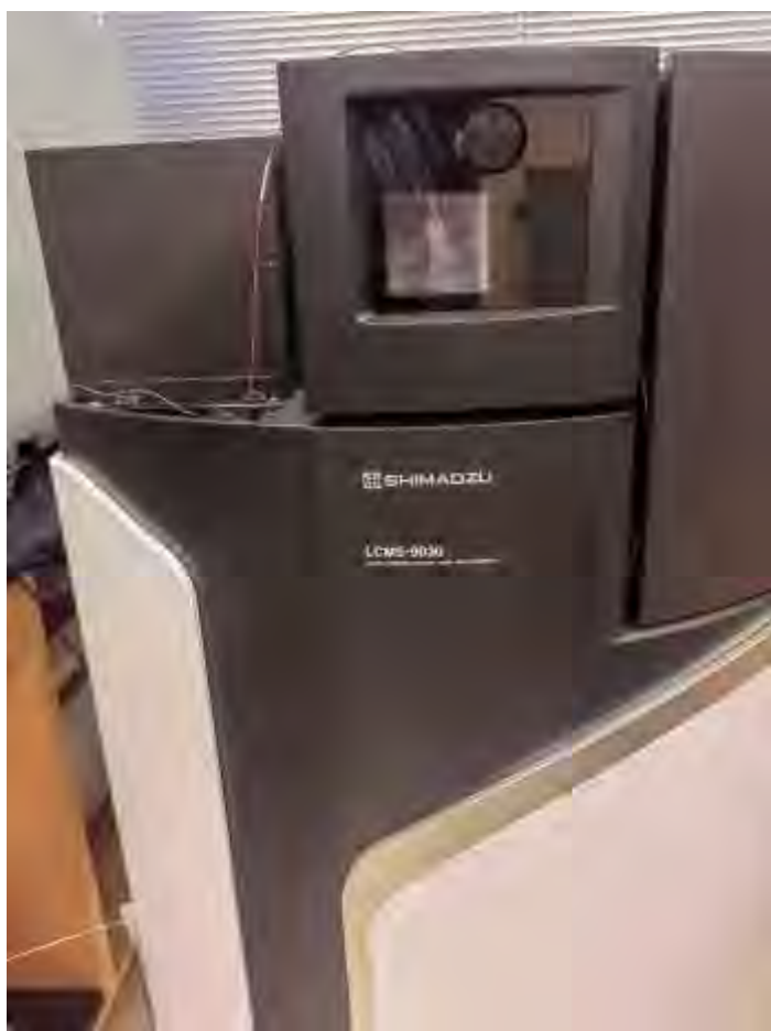
Figure 4. A tour of the lab to see cutting-edge laboratory equipment. The LCMS-9030 quadrupole time-of-flight (Q-TOF) mass spectrometer is a powerful instrument that integrates the world's fastest and most sensitive quadrupole technology with TOF capabilities for accurate mass measurement. We intend to use the equipment for our metabolomics experiments.
